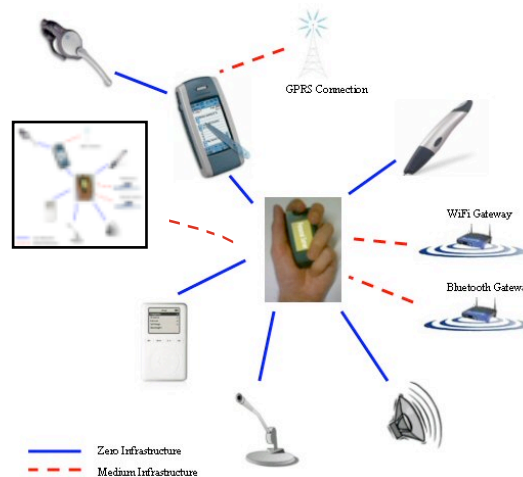
Fig. 1. Task-aware context and data plane services running on personal server. This controls the available input and output modalities for set of task functions running in the Personal Area Network (PAN) or the Personal Local Area Network (PLAN), respectively.
